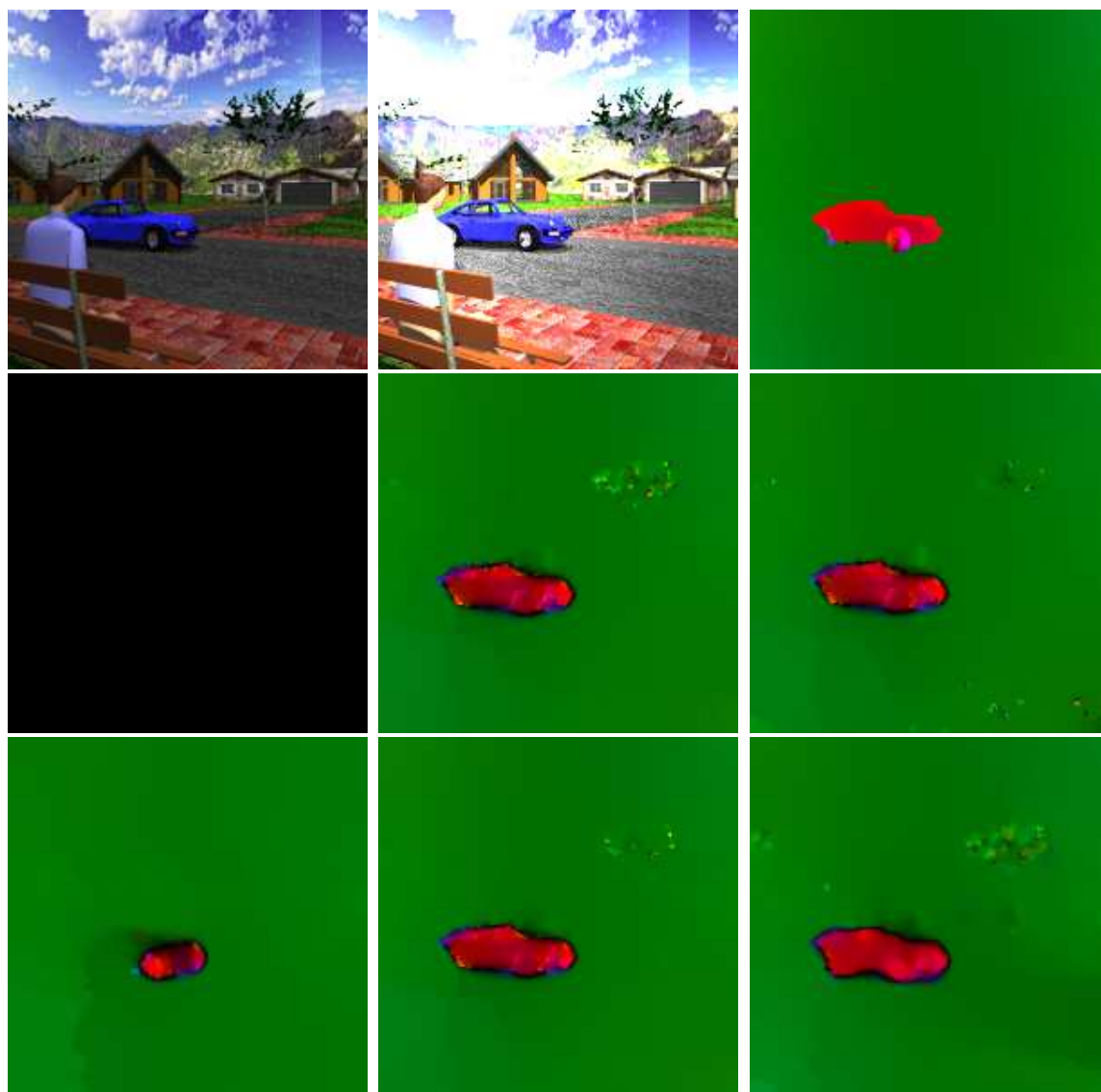
Figure 6.14: Experiment 2.II: Multiplicative illumination changes Top Left: Frame 10 of the “Street” sequence; Top Center: Frame 11 (with multiplicative illumination changes); Top Right: The ground truth colour-coded flow field between frame 10 and frame 11; Middle Left: The colour-coded flow field, computed with the Brox et al. multichannel method for the RGB constancy assumption; Middle Center: The arithmetic mean assumption; Middle Right: The geometric mean assumption; Bottom Left: The hue assumption; Bottom Center: The \phi\theta assumption; Bottom Right: The log-derivatives assumption.
