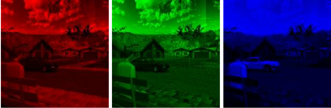
Figure 3.4: Left: the red channel for frame 10 of the “Street” sequence; Center: the green channel; Right: the blue channel
