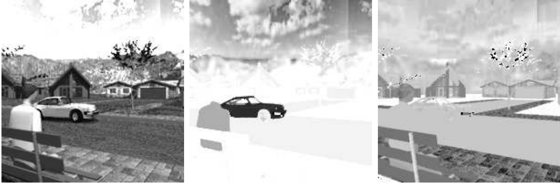
Figure 3.9: The \tau\phi\theta channels: black-and-white coding. Left: the \tau channel for frame 10 of the “Street” sequence; Center: the \phi channel; Right: the \theta channel.
