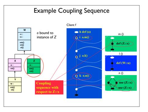
A coupling sequence is a sequence of method calls in which a variable shared by a common instance context is defined in one method and used in another method.
