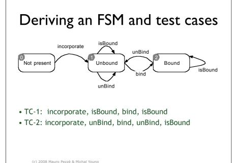
A simple analysis of the informal specification of class Slots allows to identify states and transitions. This state machine allows to derive sequences of method calls for intra-class testing, for example by choosing method call sequences that cover all states or transitions in the FSM.
